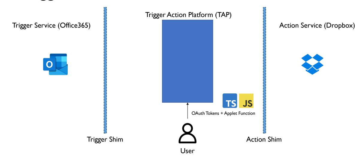
Trigger Action Platform (TAP) Trigger Service (Office365) Action Service (Dropbox) Interpreter/JIT **Applet Function** (Does email subject contain "IFTTT"?) OAuth Tokens + Applet Function Trigger Shim **Action Shim** User
