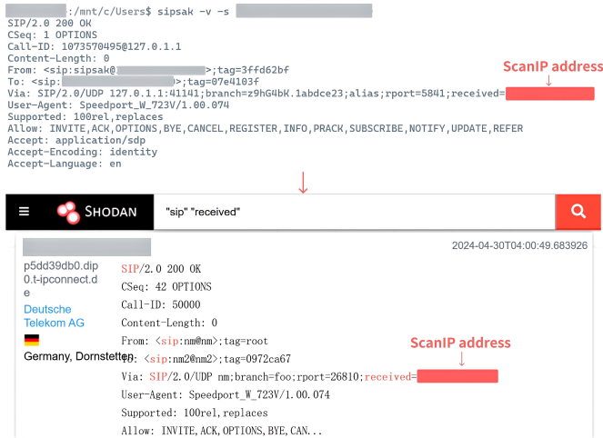
Fig. 1: IP Mirror Service. Interacting with a SIP server by sipsak -v -s {IP} will reply with the sender’s IP. When querying {"SIP" "received"} in Shodan, its ScanIP is shown under the red mark.
