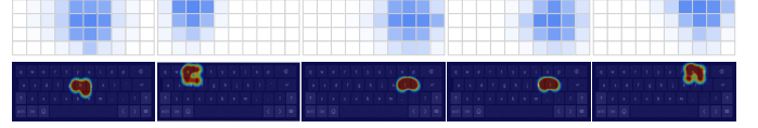
Fig. 8: Keystroke heatmap generation when the VR user types the word “HELLO” on the virtual keyboard. Upper part: confusion matrices of extracted IR features. Lower part: generated heatmaps on the virtual keyboard (§ IV-D).
