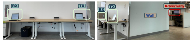
Fig. 22: Experiment Settings. A scenario where an adversary sends an adversarial signal from behind a wall in LoS Tx-Rx.
