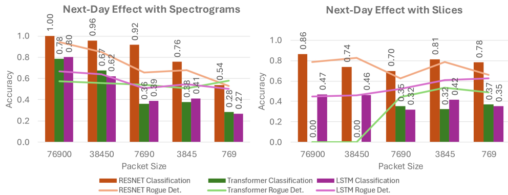
Fig. 9. Effects of training feature extractor models with Day 1 data for classification and rogue device detection with Day 2 data - Next-Day Effect.
